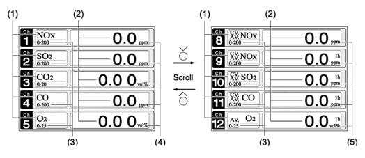
Scroll the UP and DOWN keys to display more than 5 channels.
